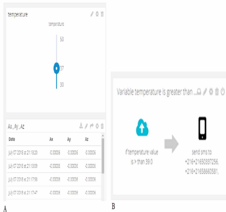
Figure 11. A) Temperature and acceleration display on the dashboard, B) event part in Ubidots
