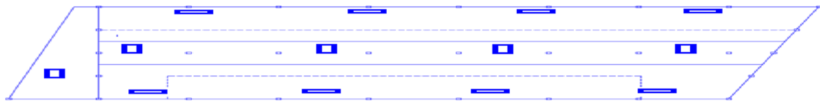
Figure 3. Industrial Electric Heater Placing
