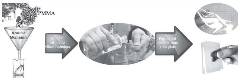
Figure 5. Schematic diagram showing the solution casting on glass technique for the preparation of the ionogel film.
