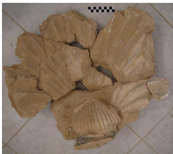
Figure 15. Shell of lime mortar coming from the house H10. Condition before conservation (Photo W. Osiak)
