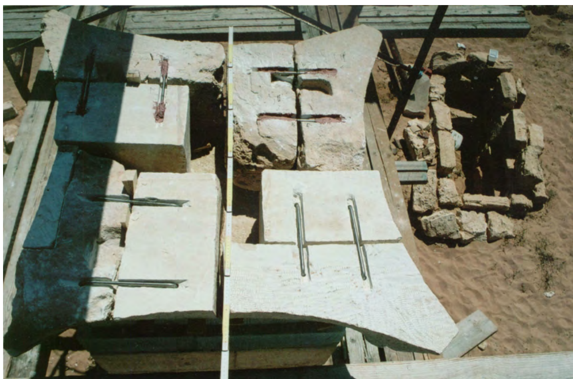
Figure 3. Anastylosis of a pillar of tomb T12: layout of blocks in the capital layer with clamps fastening pairs of stones together visible. (Photo W. Grzegorek)
