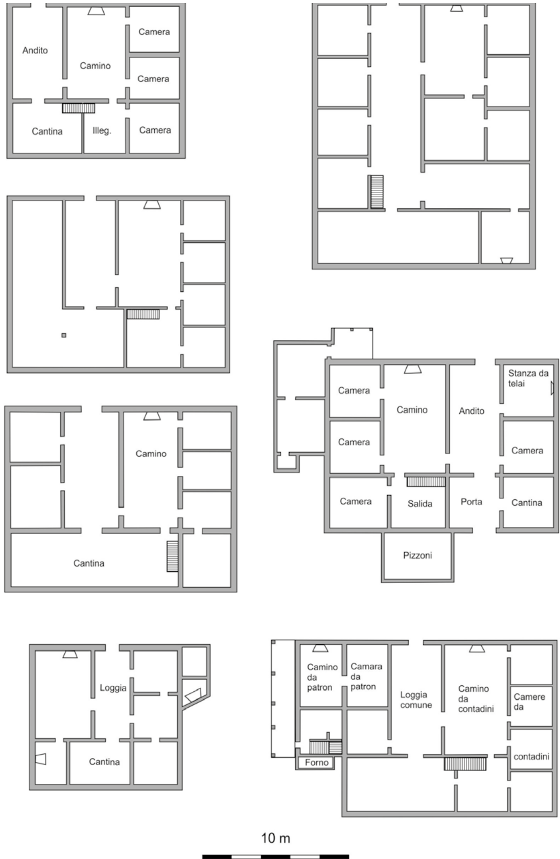
Figure 18. Plans of 17th century brick buildings, re-elaborated version based on original drawings (ASBo, Periti Agrimensori, S. Domenico, vol. 107, c. 53, a. 1650).
