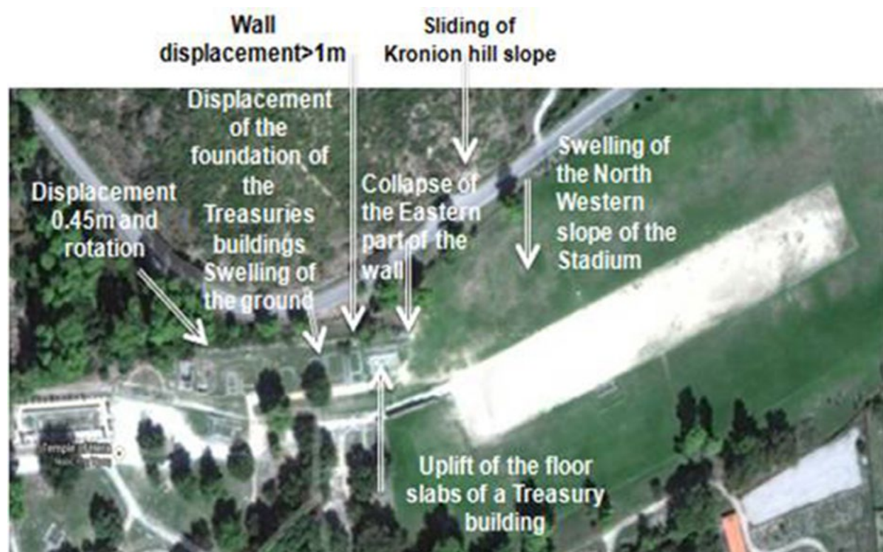
Figure 7: Overview of geotechnical instability in the wider area of the retaining wall (Google Earth view).
