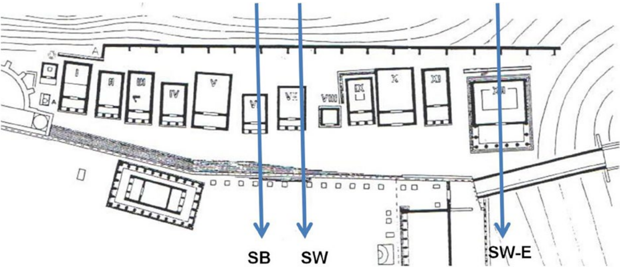
Figure 1: Plan view of the Treasuries of the Ancient Olympia sanctuary. The top wall corresponds to the retaining wall in question and protects the buildings from the Kronion Hill earth pressures (after Herrmann 1999: 368, fig. 192).
