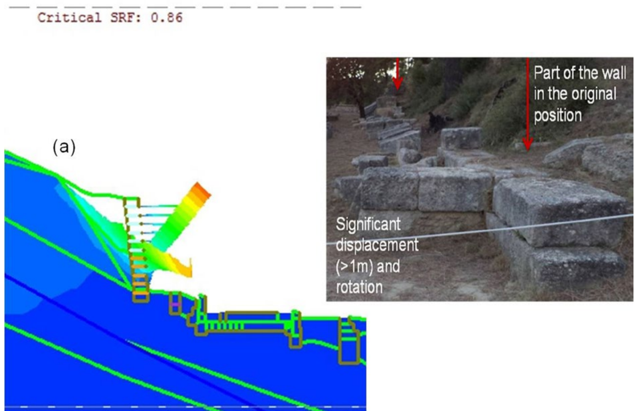
Figure 12: Results of the analytical collapse and general sliding (FS=0.86) at the eastern part of the Treasuries Wall (SW-E section). Comparison to the current state (photo: D. Egglezos).
