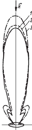
Figure 5-2: Modules of characteristics of the sound scattering of the hard spheroid
