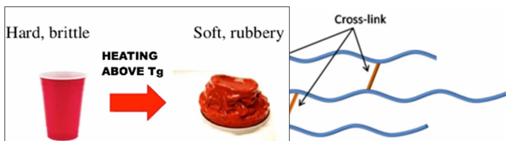
Figure 4. Effect of Glass Transition Temperature on Crystallinity/Structure
