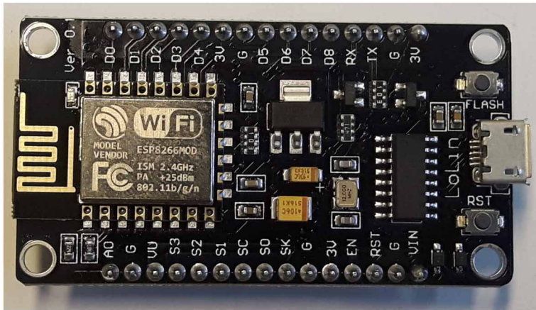
Figure 3. An electronic board capable of communicating via WiFi with nearby smartphones or directly to the Internet. An antenna is visible at the left side, a USB port at the right side, and at the top, the bottom is a series of pins allowing connection of inputs and outputs. The device is equipped with a microcontroller capable of being programmed to perform specific tasks — device with about 8 cm.
