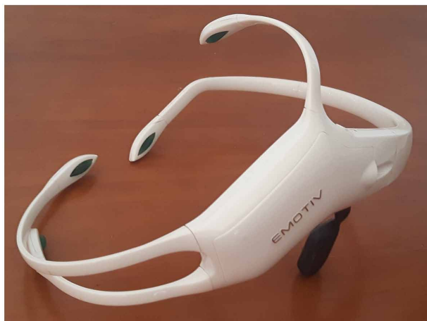
Figure 1. A commercial portable EEG device capable of communicating via Bluetooth with the mobile phone
