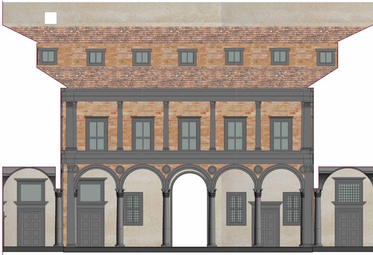
Figure 5. The elevation represents the medium LOD of the courtyard that corresponds to a scale 1:100
