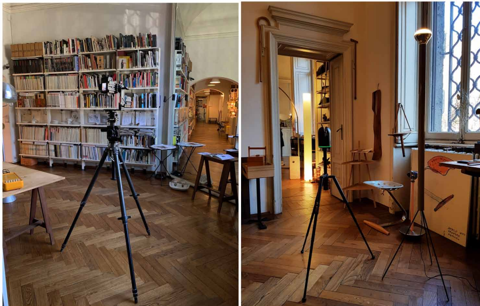
Figure 5. Instruments used: on the left, Canon EOS 70D camera mounted on a tripod with a panoramic head; on the right, laser scanner Leica BLK360
