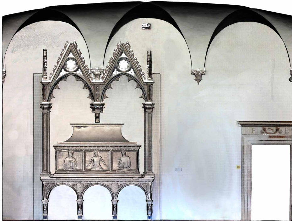
Figure 2. Slice of the point cloud: section shows the survey accuracy in one of Duca's apartment room with a coffin
