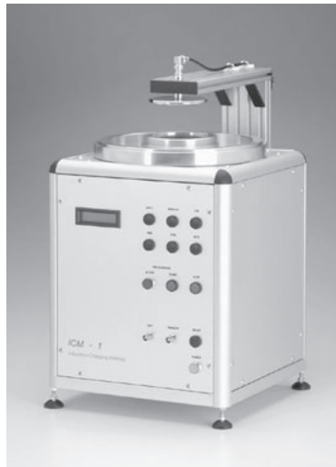
Figure 5.3. The measuring device ICM-1 (for induction charging method)
