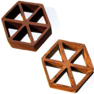
Fig. 8.17: Cermet honeycomb structures before (left) and after (right) the service life testing [29].
