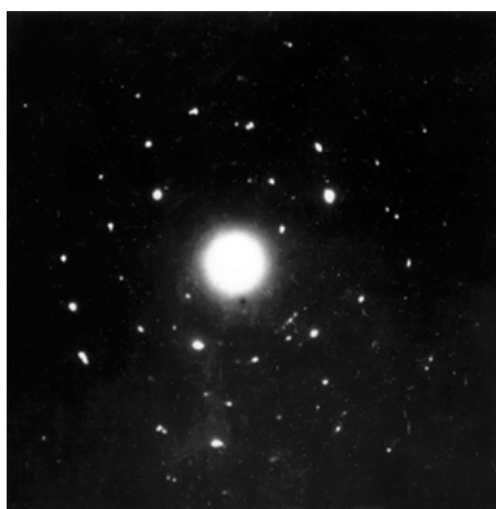
Fig. 6.6: Microdiffraction from the \text{LaFeO}_3 sample calcined at 900 °C.
