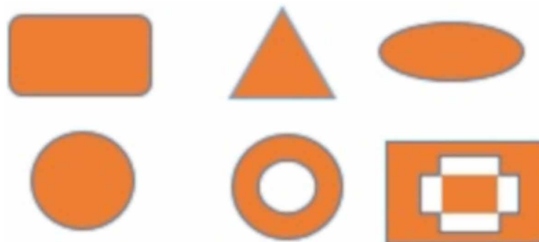
Figure 2. Arbitrary Patch Microstrip Antenna different Patch Shapes
