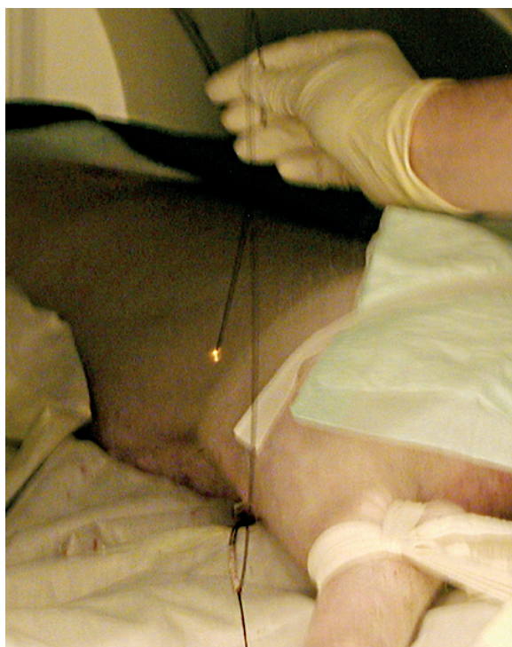
Fig. 3.65 Heating of a nitinol wire. During ongoing MR measurement, bending the tip of a commercially available nitinol wire when touching the pig caused sparks to form on the end of the wire.
