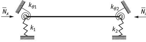
Fig. 6.6: A typical laminated composite columns under axial compression having spring-based boundary conditions. 7
