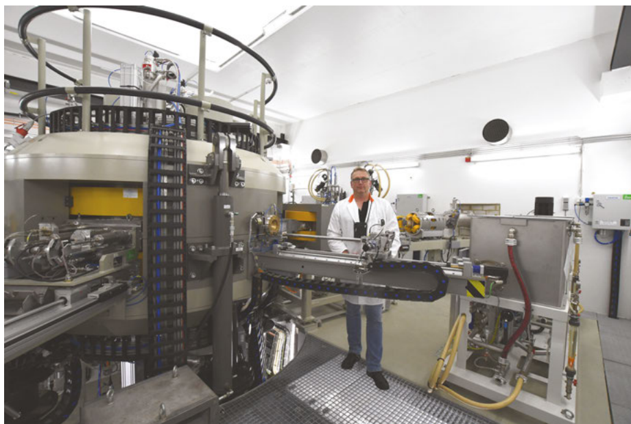
Photograph: Partial view of the IBA Cyclotron CPX 30 at the Forschungszentrum Jülich (courtesy FZ Jülich).
