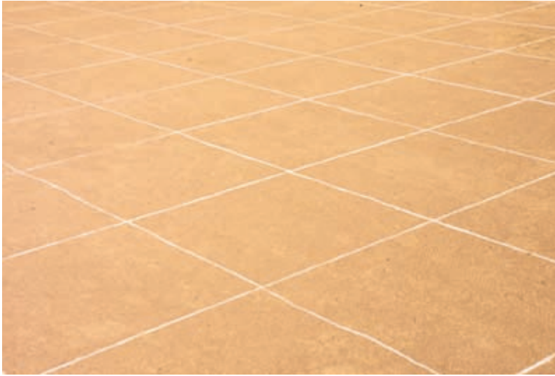
1.4 View onto a test field provided with a grid of 1 m squares painted on the flat and barren desert floor
