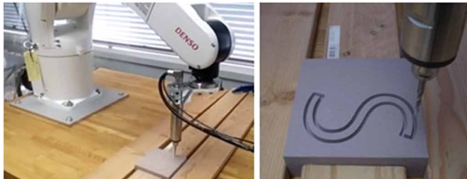
Figure 19. Machining scene of an outline font using an industrial robot VS068 with ORiN middleware, in which the desired trajectory of the small ball-end mill is a CLS file made from the outline font drawn by using Adobe Illustrator
