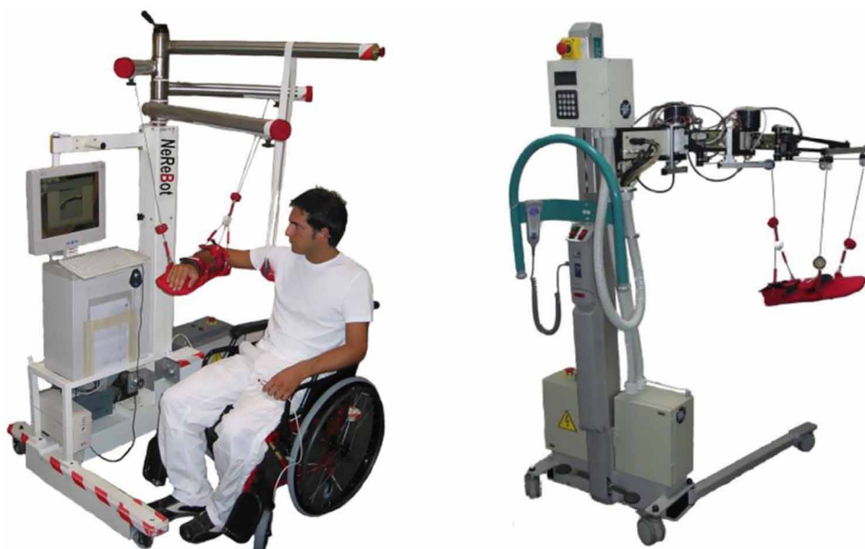
Figure 16. Cable-driven robots: (a) NeReBot; (b) MariBot (Rosati et al., 2017)
