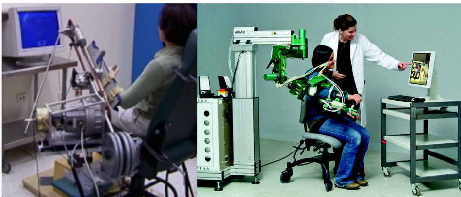
Figure 11. Robotic system for arm rehabilitation: (a) ARM; (b) ARMIN (a) (Kahn et al., 2001); (b) (Novak et al., 2015)
