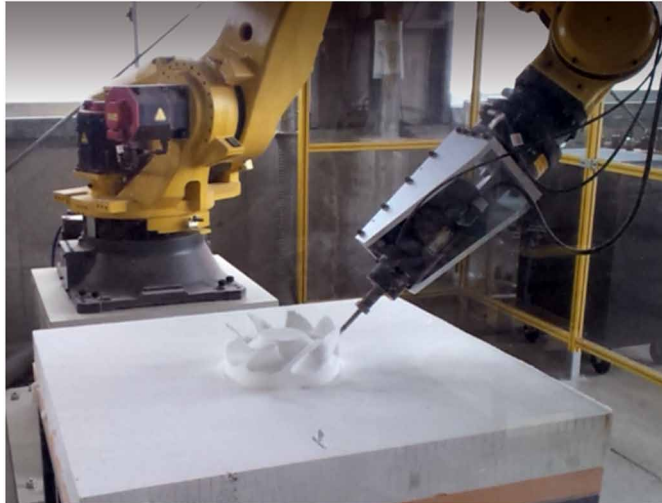
Figure 1b. Presents machining scene of an impeller model using FANUC R2000iC industrial robot (SOLIC Co. Ltd., Japan)
