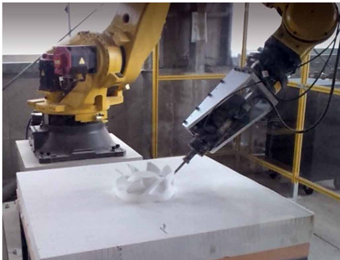
Figure 22. the output of the CAM model in Fig. 21 is applied to machining of a foamed polystyrene using an industrial robot FANUC R2000iC
