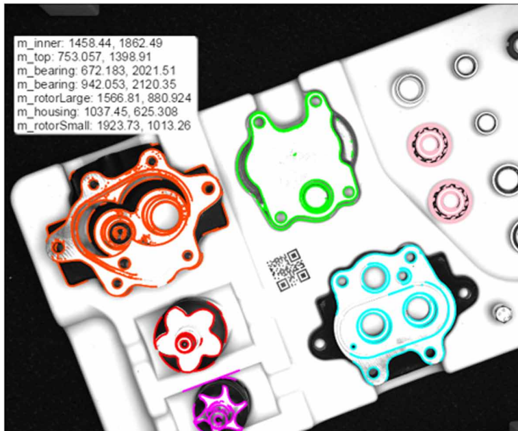
Figure 7. Detecting compressor parts using machine vision
