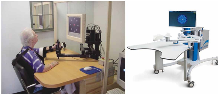
Figure 9. Rehabilitation robots: (a) MIT-MANUS; (b) InMotion ARM™. (a) (Krebs et al., 2003); (b) (InMotion, 2018)
