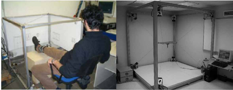
Figure 13. Cable-based robots: (a) CALOWI; (b) MACARM
