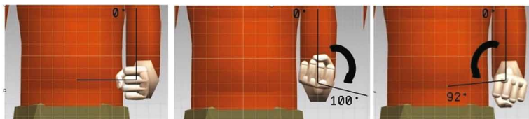
Figure 6. A CAD model for forearm pronation-supination measurements: (a) initial position; (b) upper limit; (c) lower limit
