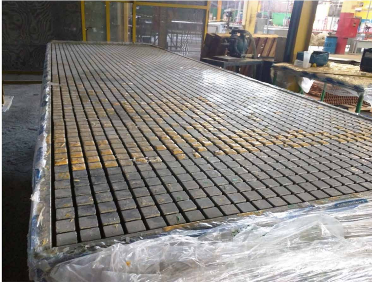
Figure 4. FRP gratings table with mold (produced by the authors)
