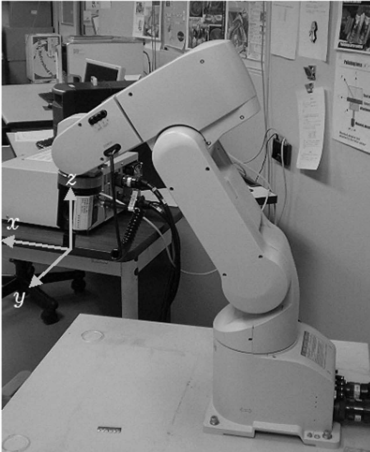
Figure 1a. Shows articulated industrial robot with an open architecture controller
