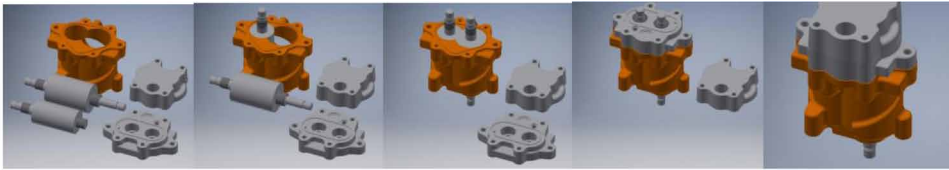
Figure 9. Assembly sequence of the main parts. From left to right: unassembled - small rotor inserted - both rotors inserted - middle lid added - top lid added
