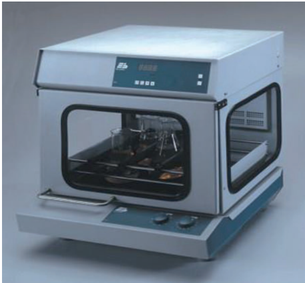
Figure 6.3: Set-up of a standard shake flask method for determining solubility.
