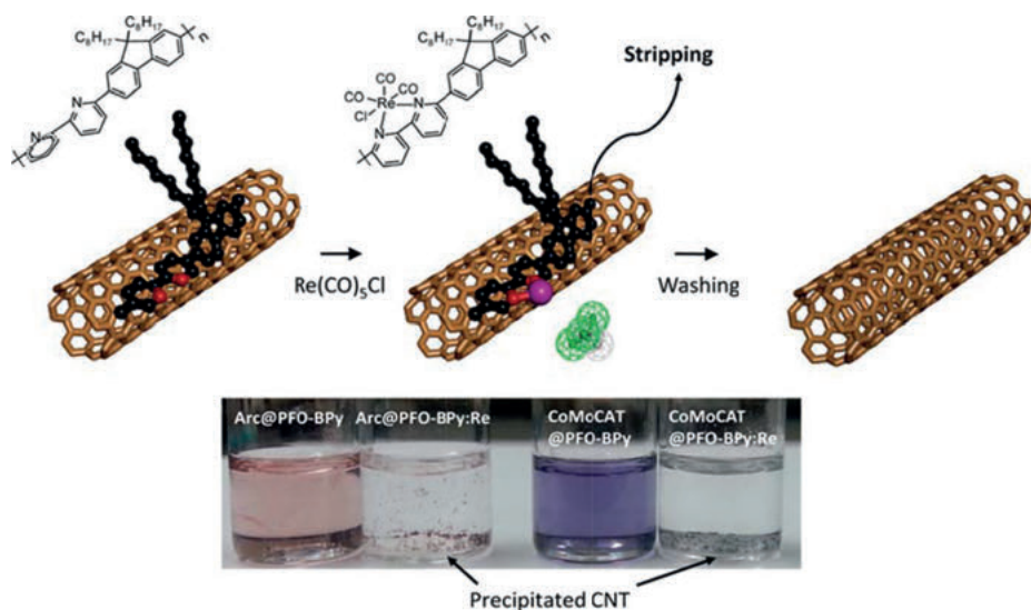
Figure 13.2: Schematic illustration of the process used to produce pristine sc-SWNT by removing wrapped polymer from SWNT surface by complexation with Rhenium complex. Images of solutions of polymer-wrapped s-SWNTs before and after the reaction with \text{Re}(\text{CO})_5\text{Cl} . Reprinted with permission from Ref. [17]. Copyright 2018, American Chemical Society.
