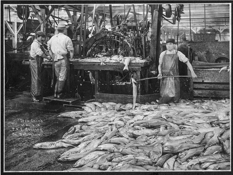
Fig. 4 “Iron Chink” cleaning machine in operation with Asian worker at the Pacific American Cannery, Fairham, Washington, ca. 1911–1913. University of Washington Libraries, Special Collections, UW 39788.
