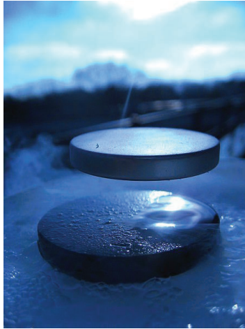
Photo of magnetic levitation, using high temperature superconductor \text{YBa}_2\text{Cu}_3\text{O}_7 at the bottom. 7
