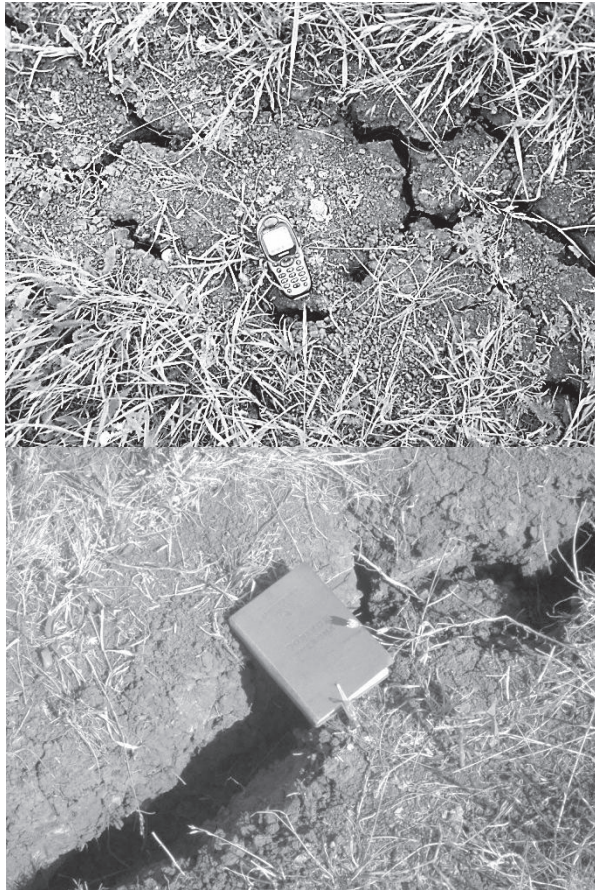
Figure 1.2.6: Cracking of the soil at the North Stavropol GSF site and the Pelagiadian structure in August 2001.
