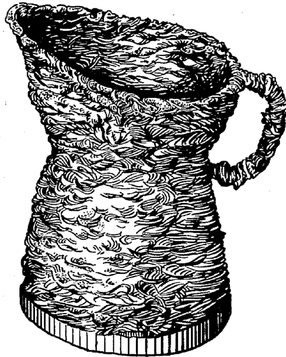
Figure 1. A jug fabricated from metal using layer-by-layer arc-welding according to a 1925 patent 1 assigned to Westinghouse
