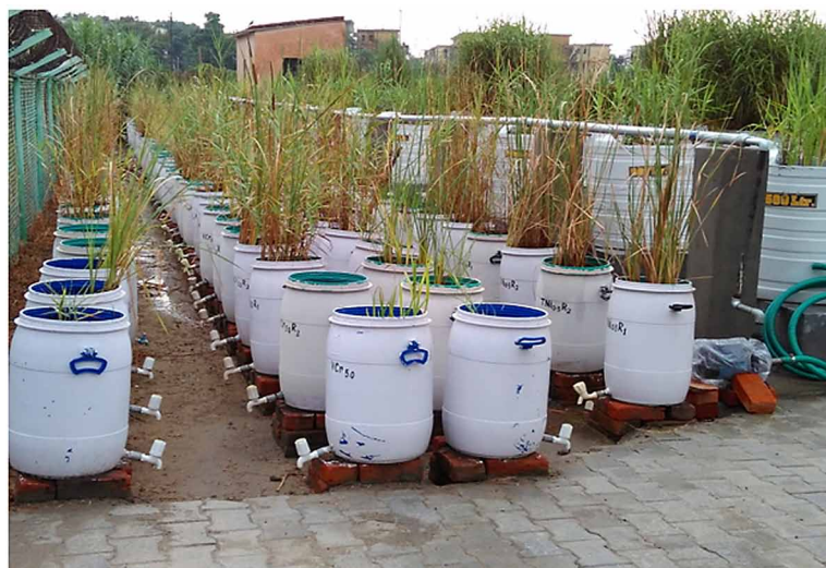
Figure 1. A view of the vertical subsurface flow constructed wetlands of IARI
