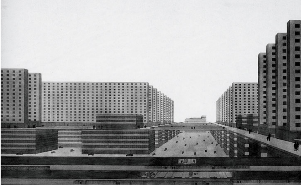
Ludwig Hilberseimer, Hochhausstadt project, east–west street view, 1924. Perspectival drawing that highlights the division of urban circulation while visualizing how architectural volumes penetrate and connect the different layers of transportation.
