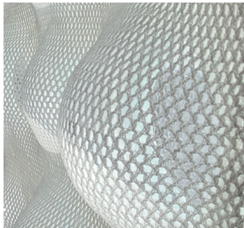
Varying transparency of a 3D textile by stretching the deck layers perpendicular to each other
