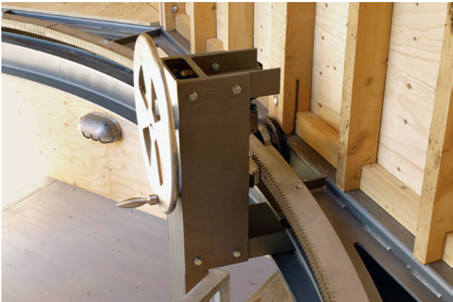
Drive: hand-operated wheel with geared cogwheel and radial rack
