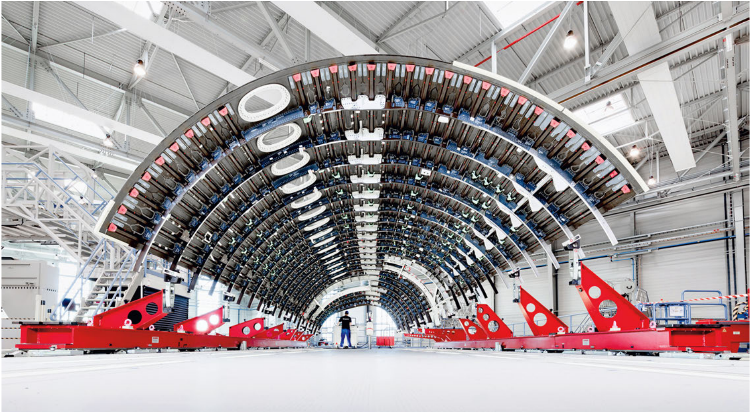
CFRP fuselage shell of an Airbus A350
