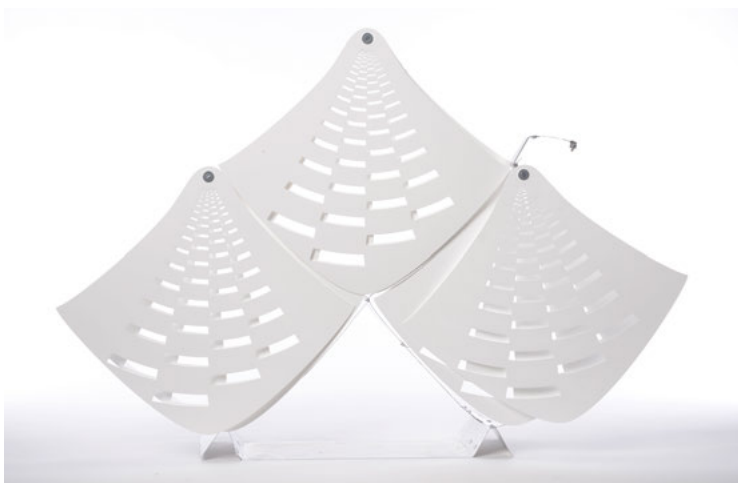
Overlapping shifting elements employing a shape-memory coil spring actuator to produce a translation movement – shown here in the open state (left) and the closed state. The demonstrator is known as “Chameleon Membrane”.
