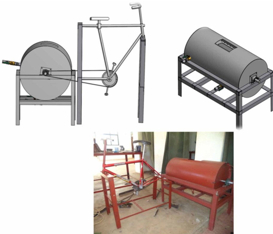
Figure 9. 3D CAD model and picture of the fabricated pedal-driven washing machine
