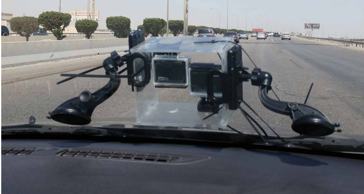
Figure 7. An example showing two GoPro cameras attached to a car's hood, to record the journey and then produce a 3D movie
