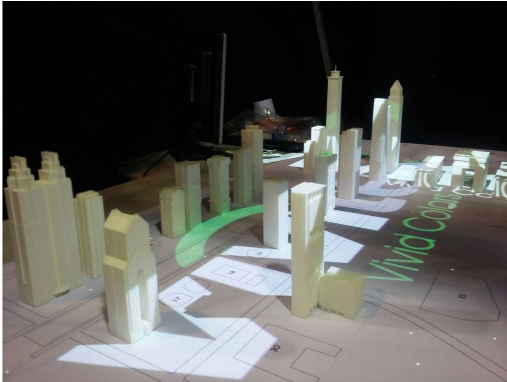
Figure 5. A simplified scale model of the city of Dubai during one of the projection tests performed to setup the multi-projector SAR application
