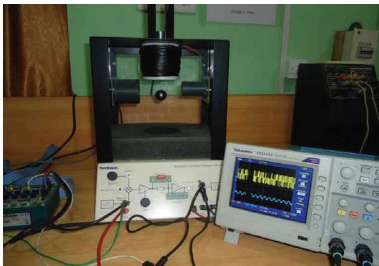
Figure-P2: Picture showing magnetic levitation where classical calculus is used for controls
