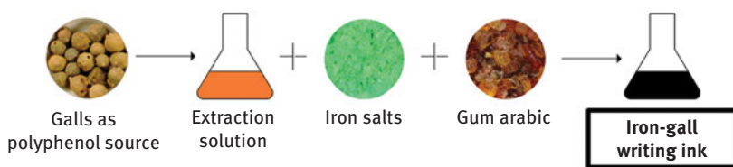
Figure 16.5: Main steps and ingredients in the production of iron gall ink: an extract solution from galls, to which iron sulphate is added, forming a black precipitate. Gum arabic is added to keep the precipitate in suspension.
