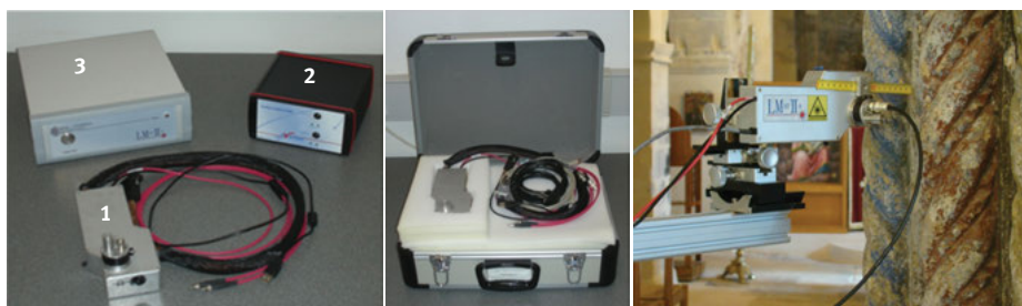
Figure 4.5: Main subunits of LMNT-II+ (left) and instrument in carrying case (right).
