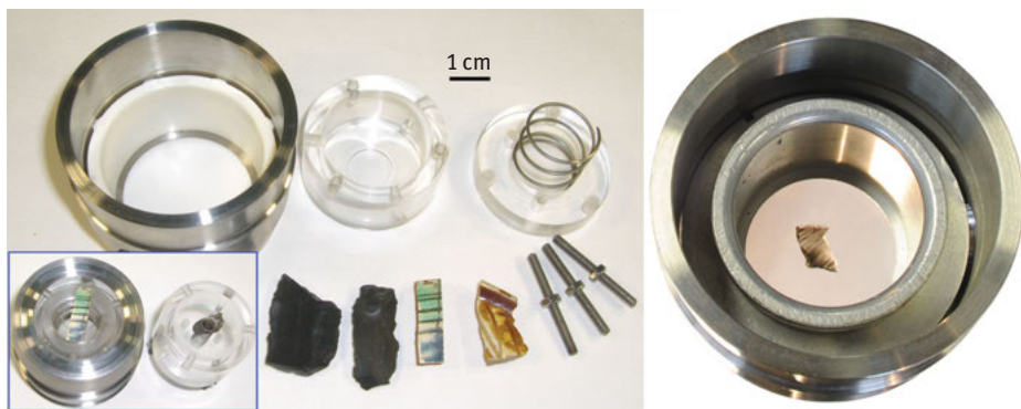
Figure 2.13: WD-XRF spectrometer sample holder equipped with plexiglas capsules in which the samples (two obsidians and two pieces of ceramic) can be fixed (see the inset in the left lower part of the figure); the plexiglas boxes were built with different diameter holes through which the more regular surface of the artifacts can be exposed to the spectrometer X-ray source. On the right the WD-XRF sample holder closed at the bottom with a very thin Mylar® polyester film on which a little obsidian specimen is placed, as suspended in the air.
