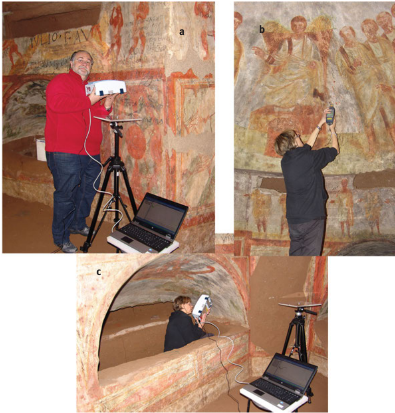
Figure 11.1: Some examples of data acquisition with portable instruments in the Domitilla's Catacombs. (a) and (c) FT-IR TR; (b) XRF. Photos by Giovanni Bartolozzi.
