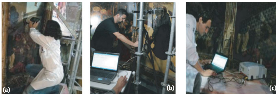
Figure 15.10: Snapshots of in-situ analyses performed during the Funchal altarpiece study. (a) colorimetry, (b) EDXRF, (c) p-FTIR.
