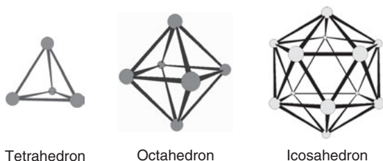
Figure 2.13: Polyhedrons of particularly high symmetry (PLATONIC solids): tetrahedron with 24 symmetry operations ( 8C_3 , 3C_2 , 6S_4 , 6\sigma_d , E ); octahedron with 48 symmetry operations ( 6C_4 , 8C_3 , 6C_2 , i , 8S_6 , 6S_4 , 3\sigma_h , 6\sigma_d , E ); icosahedron with 120 symmetry operations (e.g., 12C_5 , 10C_3 , 15C_2 , i , ...). A cube also belongs to point group O_h .
