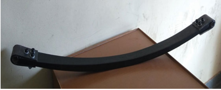
Figure 1.11: Composite leaf spring with eye joint (varying W , T ).
