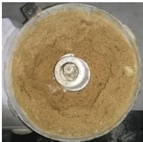
Figure 5.1: Soy meal adhesive (SMA) after mixing the constituents.
