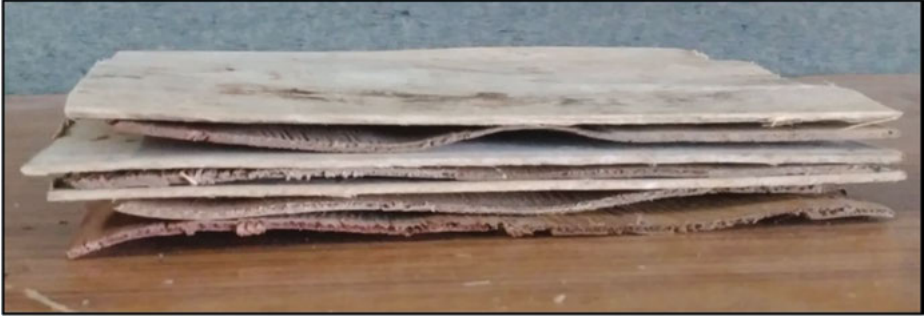
Figure 5.2: Seven stacked-up veneers.
