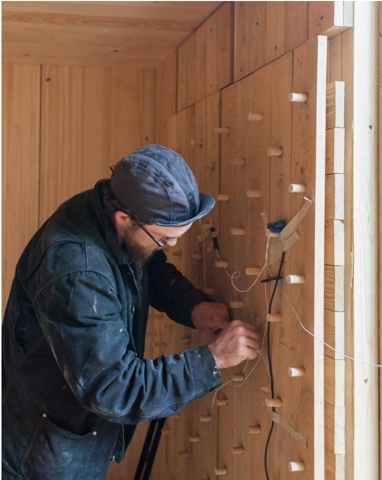
Figure 2. TLT heat flux sensor setup, April 2016
