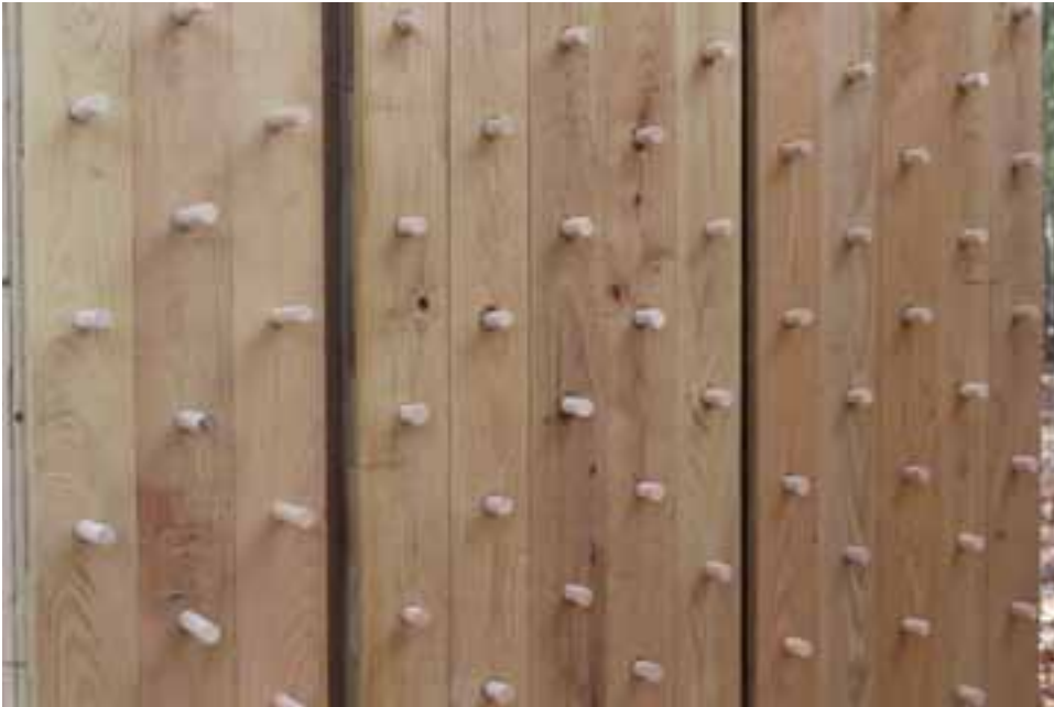
Figure 6. Thermally tuned mass timber panel from TLT, May 2016
