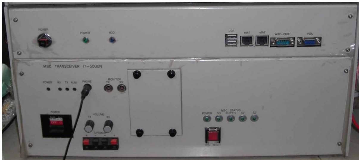
Figure 9b. Two types of transceiver developed by the author's research group: IT-5000N (powered by SBC)
