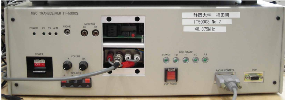
Figure 9a. Two types of transceiver developed by the author's research group: IT-5000S (powered by DSP)
