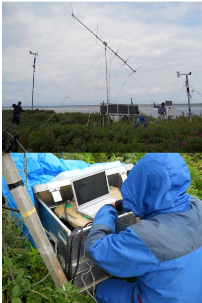
Figure 2c. Lake Saroma remote station: Upper; System overview and Lower; backup scene from data logger to note PC. The data logger is installed in a duralumin box
