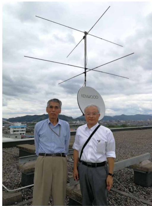
(b) 2-element cross Yagi-Uda antenna set elevation angle as 90 degrees for transmitting the beacon carrier at 53.750 MHz. The Left side is Professor Maegawa and the right side is the author.
