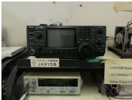
Figure 10. The beacon carrier transmitting system for HRO of JA9YDB in Fukui National College of Technology. The photographs were taken in Sept. 12, 2019
