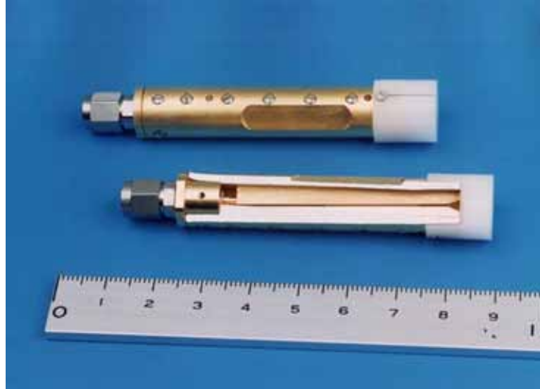
Figure 10. Ultra-broadband double ridged horn antenna with small aperture, developed for active phased array antenna
