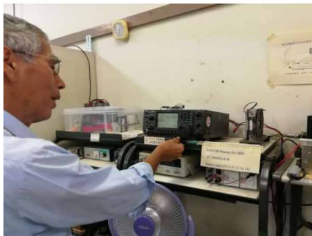
(a) The beacon carrier transmitting system for HRO in JA9YDB. The IC-7400 made by ICOM Inc. is used for transmitter.
