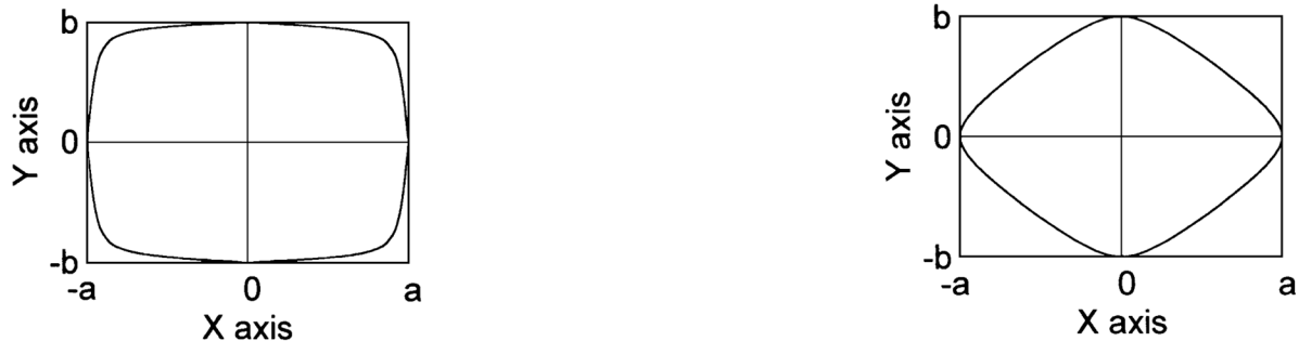
Figure 8. Scattering pattern by caustic corrected expression: \theta -polarization, \phi_0 = 0^\circ , solid line: caustic correction, diamond \diamond : numerical integration
