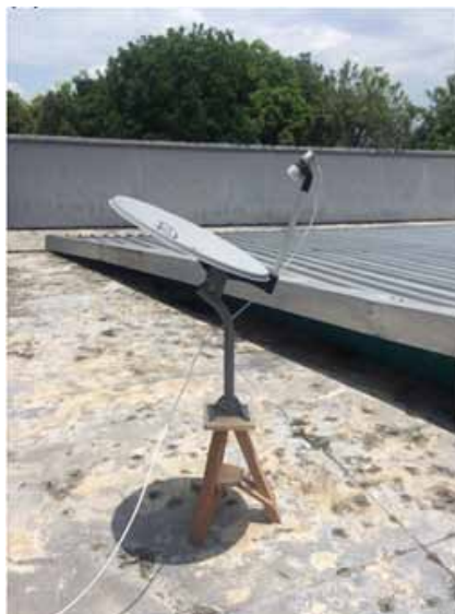
Figure 7. The off-axis reflector antenna is supported by a tripod telescope mount
