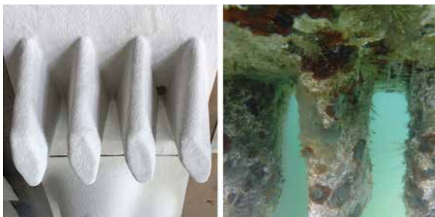
Figure 19.1. Views of ecological substrate prototype before deployment (left) and after twelve weeks underwater, colonized by invertebrate animals (right).
