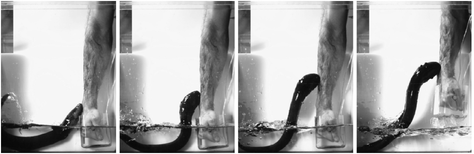
6.16. The setup for measuring the current flowing through the author's arm during an electric eel's shocking leap.
