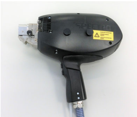
Figure 3.5: Spectrotest probe with UV-minioptics. Printed with the friendly permission of SPECTRO Analytical Instruments GmbH, Boschstr. 10, 47533 Kleve, Germany.
