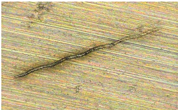
Figure 7.4: Chain of laser craters on the surface of a steel sample.
