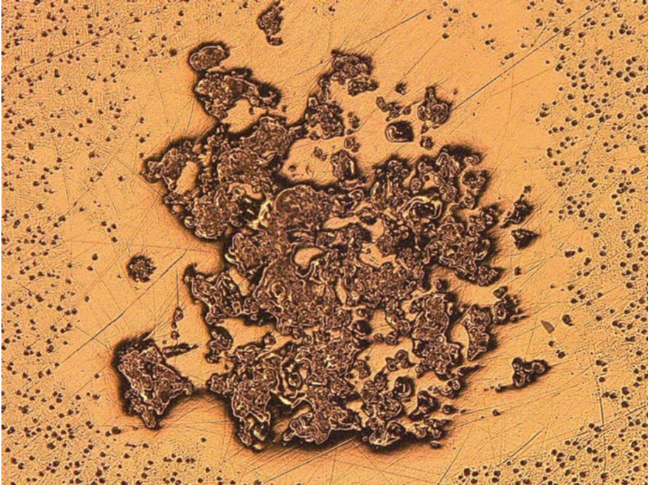
Figure 3.24: Micrograph of a gray cast sample with graphite inclusions after a 10 s pre-spark time. Printed with the friendly permission of SPECTRO Analytical Instruments GmbH, Boschstr. 10, 47533 Kleve, Germany.
