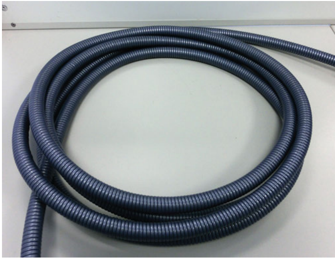
Figure 7.6: Probe hose with plastic sheath, printed with the friendly permission of SPECTRO Analytical Instruments GmbH, Boschstr. 10, 47533 Kleve, Germany.
