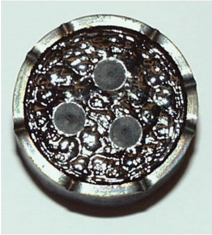
Figure 3.38: Slag sample with laser impacts. Printed with the friendly permission of Rubikon Verlag Rolf Kickuth, Bammentaler Straße 6–8, 69251 Gaiberg, Germany.
