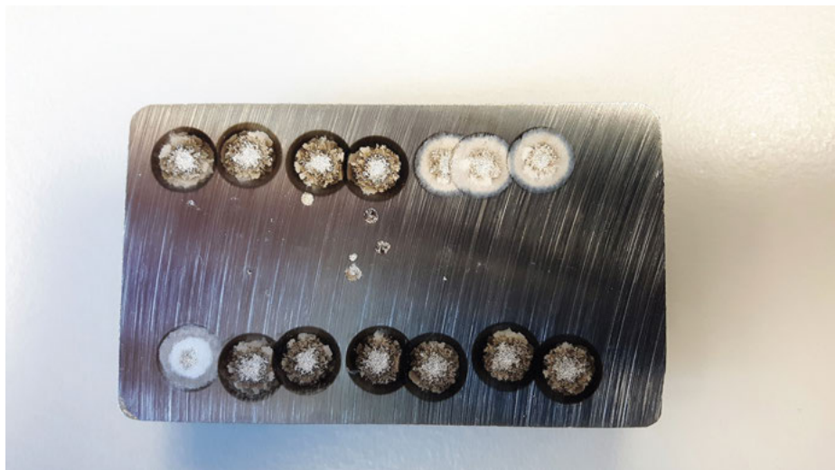
Figure 3.23: Burn spots with high (lower left) and low (lower right) fractions of diffuse discharges. Printed with the friendly permission of SPECTRO Analytical Instruments GmbH, Boschstr. 10, 47533 Kleve, Germany.
