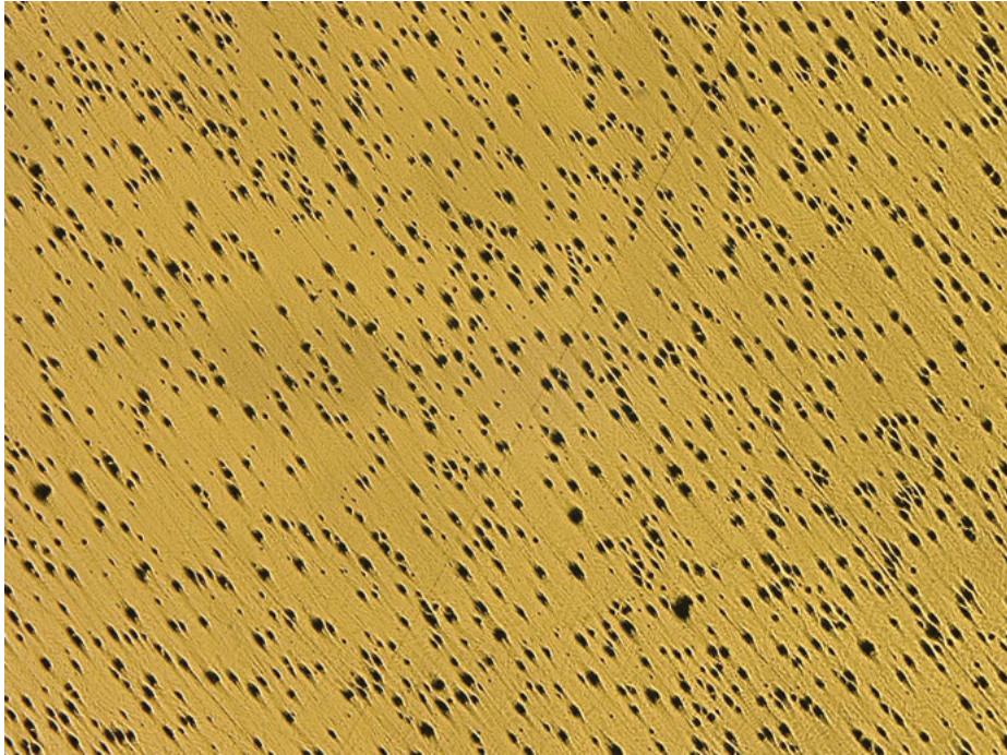
Figure 3.26: Micrograph of a sample with inclusions, scale 1:200.
