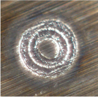
Figure 3.37: Steel sample with laser burn spots.
