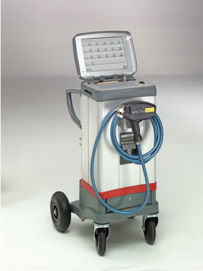
Figure 7.1: Modern mobile spectrometer, printed with the friendly permission of SPECTRO Analytical Instruments GmbH, Boschstr. 10, 47533 Kleve, Germany.
