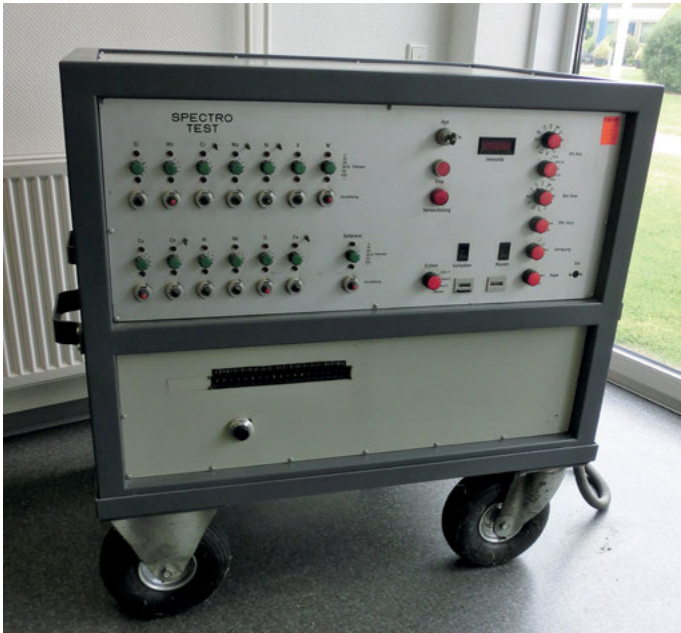
Figure 7.12: Early model of a mobile spectrometer for sorting, built in 1980, printed with the friendly permission of SPECTRO Analytical Instruments GmbH, Boschstr. 10, 47533 Kleve, Germany.
