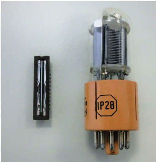
Figure 3.55: CCD chip (left) and photomultiplier (right). Printed with the friendly permission of SPECTRO Analytical Instruments GmbH, Boschstr. 10, 47533 Kleve, Germany.
