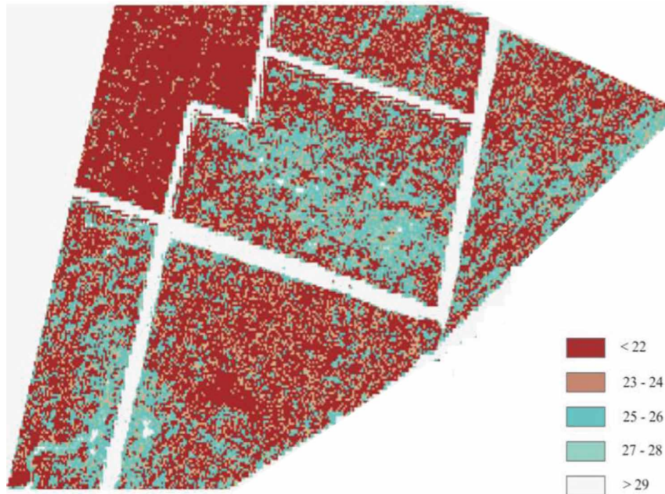
Figure 4. The map of soil humidity (%) obtained by calculation of NW
