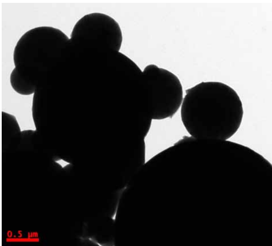
Figure 2. TEM micrograph of ferrospheres nanoparticles from fly ash
