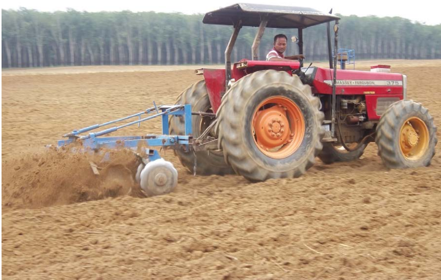
Fig. 4.6. Tractor equipped with harrow attachment.
