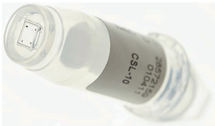
Fig. 7.3. The Alere Array Tube showing the glass slide array mounted in the base of a centrifuge tube. The oligonucleotides on the array can be seen as small spots in a square grid pattern. The larger square features on the array are used for orientation.
