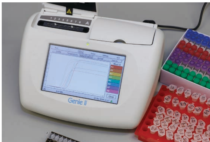
Fig. 9.3. The OptiGene Genie II instrument for real-time loop-mediated isothermal amplification (LAMP).
