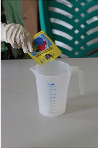
Fig. 3.4. Agar powder and sucrose are mixed in a graduated jug before cooled PSA extract is added and the volume made up to 1 litre
