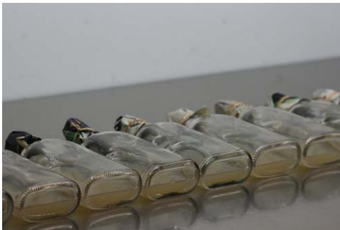
Fig. 3.9. Placement (at angle of 30 degrees) of bottles containing PSA media in laminar air flow cabinet
