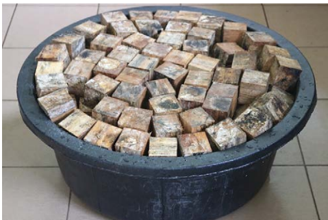
Fig. 5.9. Rubber wood soaked in water inside a big pail
