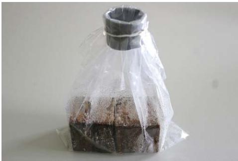
Fig. 5.11. Rubber wood blocks placed in plastic bag
