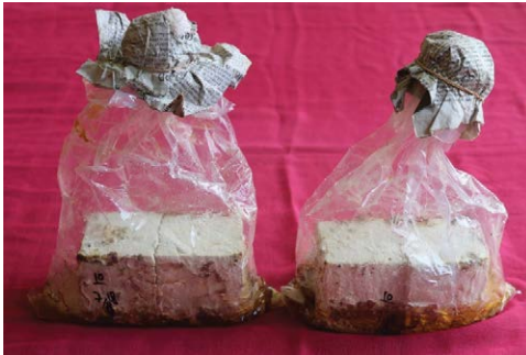
Fig. 5.16. Ganoderma inoculum on rubber wood blocks
