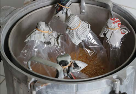
Fig. 3.11. Milled maize medium sterilization by using vertical autoclave
