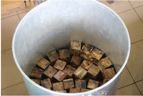
Fig. 5.10. Rubber wood blocks being boiled
