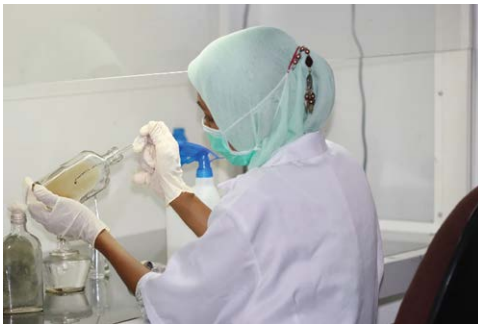
Fig. 4.2. Transfer of Trichoderma multiplication from pure isolate to PSA medium
