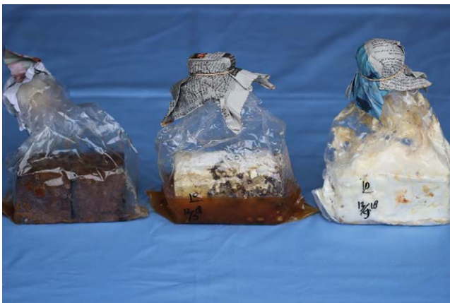
Fig. 7.5. Variation in Ganoderma coverage on RWBs from right to left high coverage (100%); medium coverage (50%) and poor coverage (<10%)
