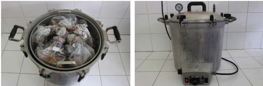
Fig. 5.13. Sterilize RWBs and PA medium using an autoclave
