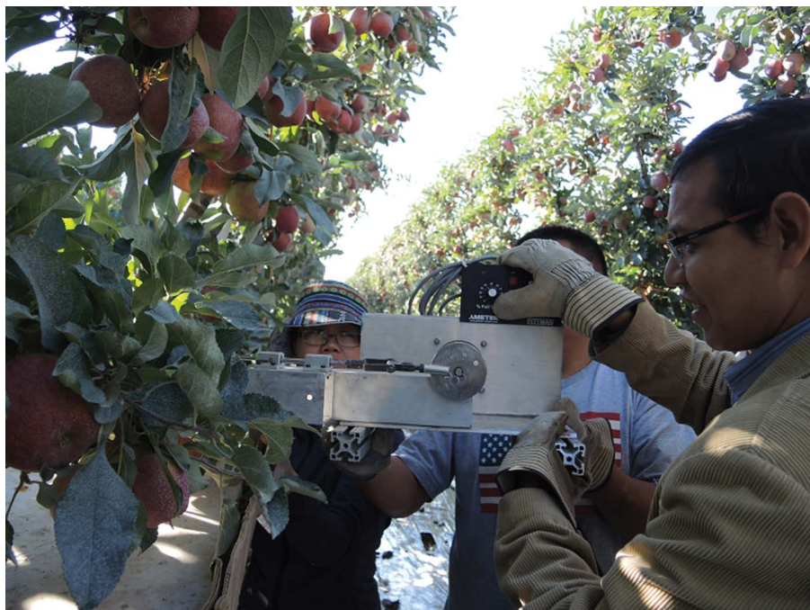
Fig. 10.10. Washington State University researchers conducting branch shaking tests in a commercial orchard using a handheld shaking device.
