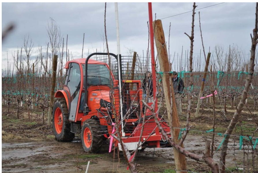
Fig. 9.4. Darwin string thinning machine mounted on a tractor.
