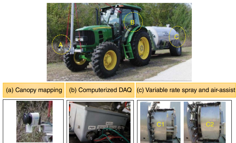
Fig. 7.2. Orchard airblast sprayer retrofitted with variable rate spray and air-assist technology; C1 and C2 represent the air-assist louver in normally closed and open position, respectively (for additional details see Khot et al. , 2012).
