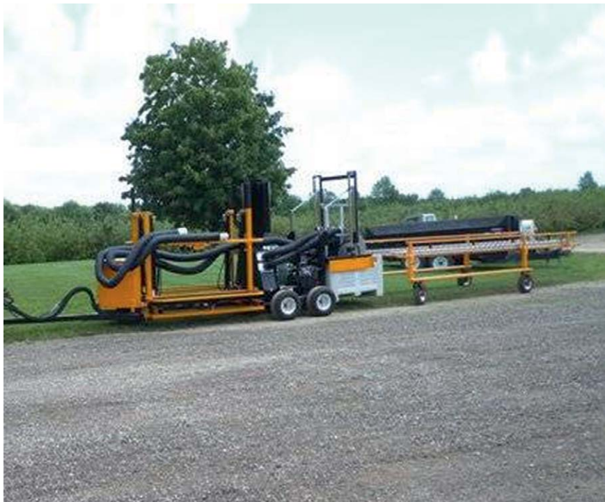
Fig. 10.13. A harvest assist machine with vacuum transportation system (from De Kleine, 2014).
