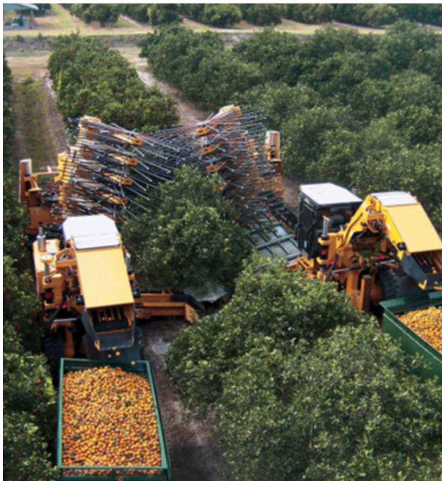
Fig. 10.9. Canopy-shaking citrus harvester Oxbo 3220 (Oxbo International Corp, from http://www.oxbocorp.com/Portals/0/Oxbo/Brochures/citrus2013.pdf ).
