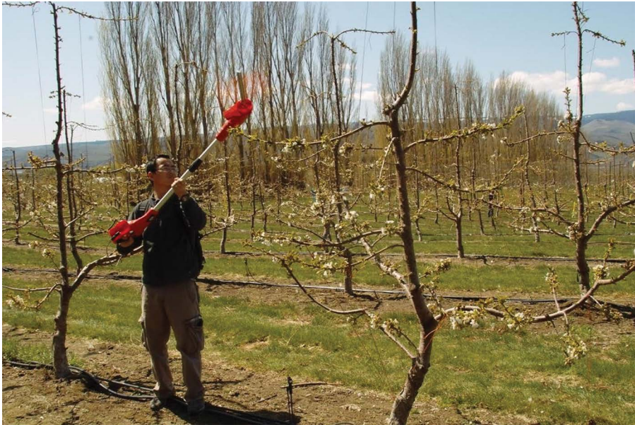
Fig. 9.5. DC-powered targeted thinning machine used in sweet cherry orchard.
