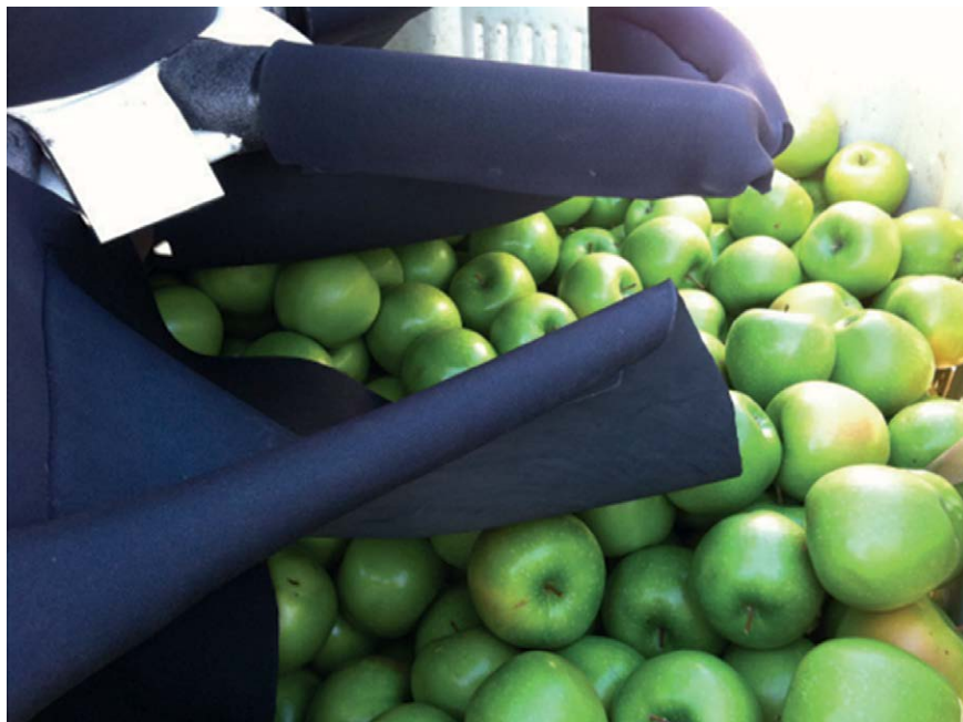
Fig. 10.14. Elephant-ear distributor in a bin-filling system (from Schupp et al. , 2011).
