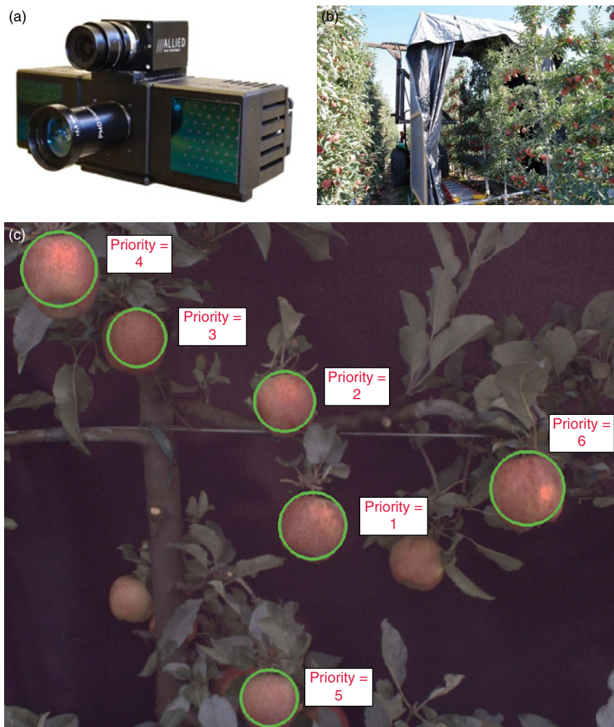
Fig. 10.19. (a) 2D and 3D camera used in vision system; (b) over-the-row sensor platform used to acquire images in a commercial apple orchard; and (c) identified apples marked by circles and picking sequence generated with Traveling Salesman Problem (TSP) (Silwal et al. , 2016a)
