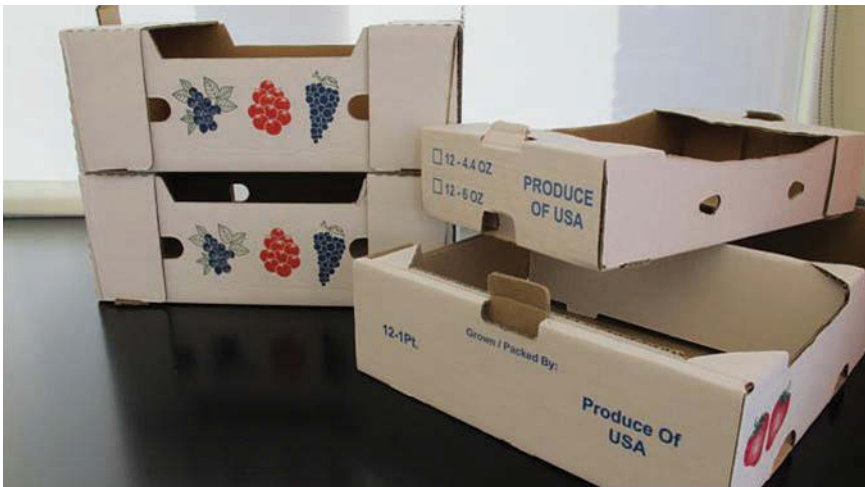
Fig. 15.5. Cardboard containers (often called 'masters' in the USA) showing reinforced corners, side vents for cooling, and interlocking tabs to help keep containers stabilized in pallet stack (P. Perkins-Veazie).
