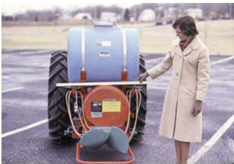
Fig. 13.19. Three-point hitch sprayer on a narrow tractor designed for spraying raspberries in narrow rows, which can apply sprays to two sides in one pass. (Courtesy: Ohio State University.)
