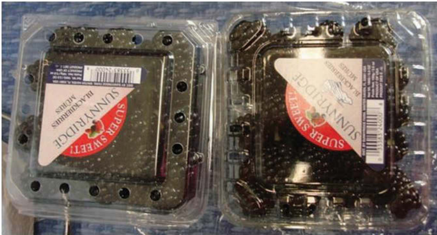
Fig. 15.4. Clamshell boxes showing holes ( left ) or slits ( right ) on top of boxes for added ventilation and cooling, and slightly elevated top of clamshell to allow for stable stacking (P. Perkins-Veazie).
