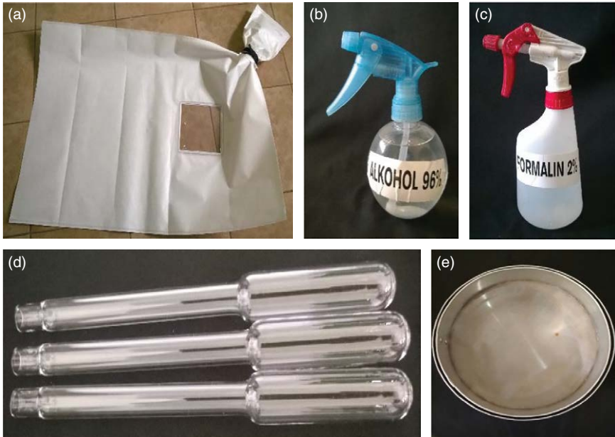
Fig. 3.2. (a) Modified isolation bag; (b) 96% ethanol in hand sprayer; (c) 2% formalin in hand sprayer; (d) ampoule glass; (e) pollen sieve.
