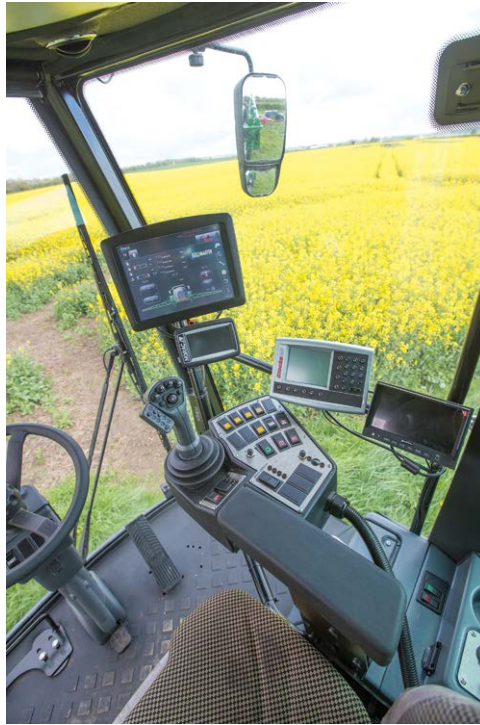
Fig. 2.9c. Modern tractor cab controls with global positioning system (GPS). (Photo courtesy of Househam.)
