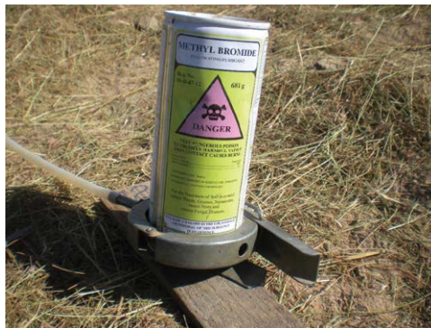
Fig. 6.6. Canister of methyl bromide ready for gas to go along tube and be released under the plastic sheet. (Photo courtesy of Kutsaga Research, used with permission.)
