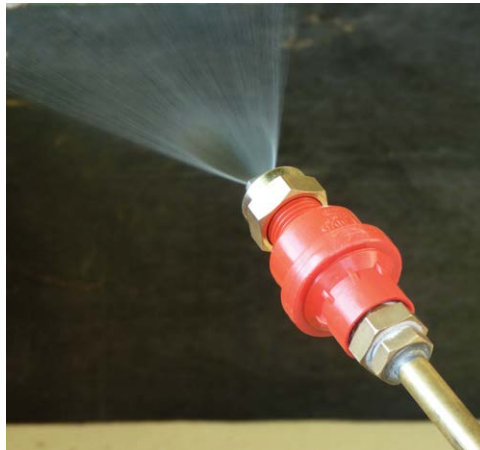
Fig. 2.8b. Fan spray with control flow valve.
