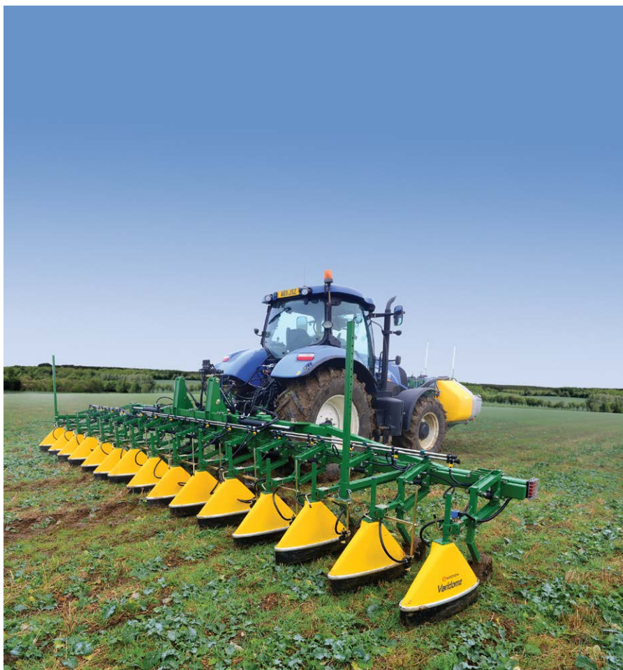
Fig. 7.5. No-drift herbicide application in inter-row application. (Photo courtesy of Micron.)
