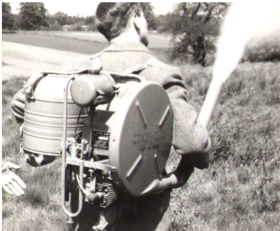
Fig. 2.16a. One of the early designs for a motorized knapsack sprayer with the fan on the side, 1957.
