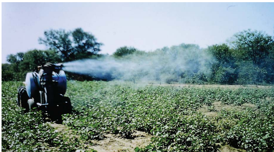
Fig. 2.15c. Misuse of a tractor-mounted mistblower treating cotton in Mozambique at noon, c.1966.
