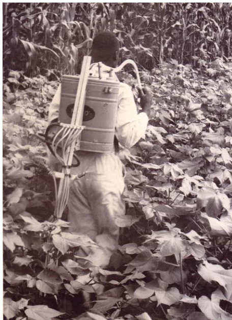
Fig. 2.7b. An early 'tailboom' being tried on a farmer's cotton field.
