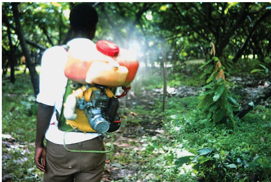
Fig. 2.16b. Motorized knapsack mistblower (Stihl), showing fan now mounted across the back of the operator.
