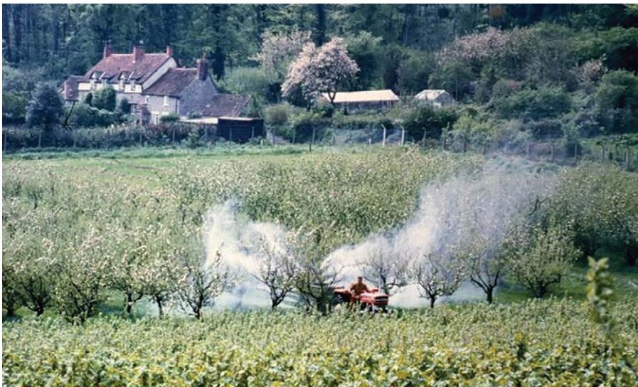
Fig. 2.14a. Orchard spraying with axial fan on the back of the sprayer to project spray through the tree canopy (Photo courtesy of Long Ashton Research Station.)
