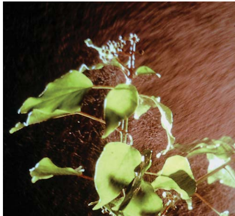
Fig. 2.19. Electrostatic spray showing movement of droplets around a single plant. (Photo courtesy of Silsoe.)
