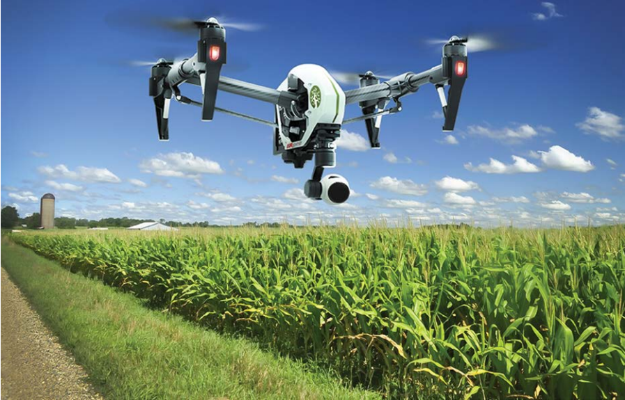
Fig. 11.1. Unmanned aerial drone with camera for collecting data on crop. (Photo courtesy of Sensat, used with permission.)
