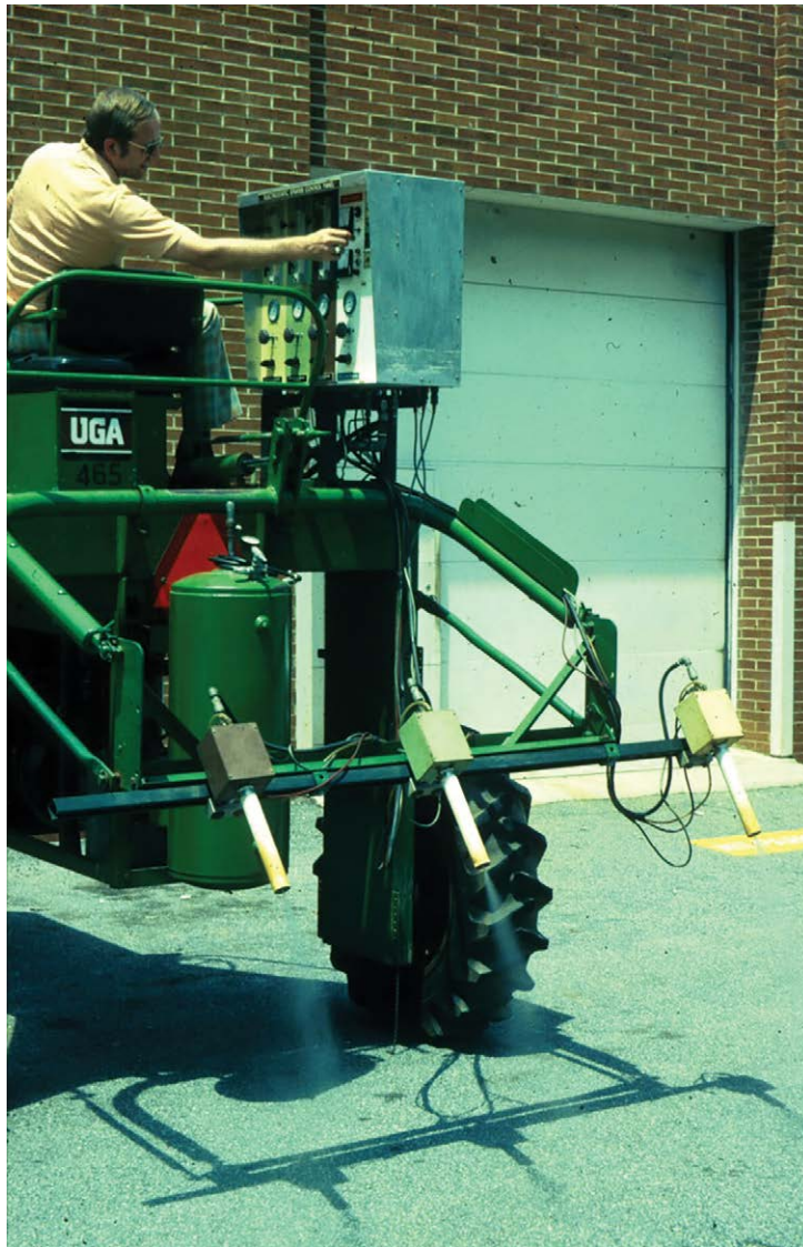
Fig. 2.21. Electrostatic spraying: Ed Law with his tractor-mounted ES sprayer.
