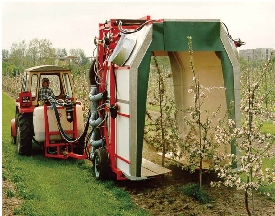
Fig. 2.14b. 'Tunnel' sprayer to reduce downwind drift of spray in an orchard.
