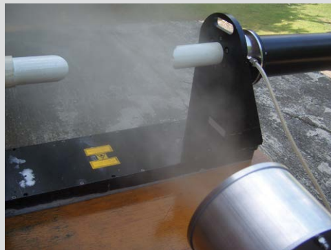
Fig. 2.3d. Measuring spray droplets using a laser system.
