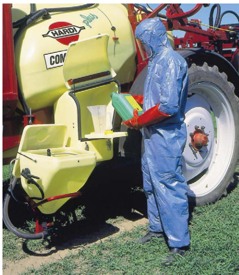
Fig. 2.11. Tractor sprayer with a low-level induction hopper to prepare sprays and a separate container for pesticide containers. Note the protective clothing worn by the spray operator. (Photo courtesy of Hardi.)
