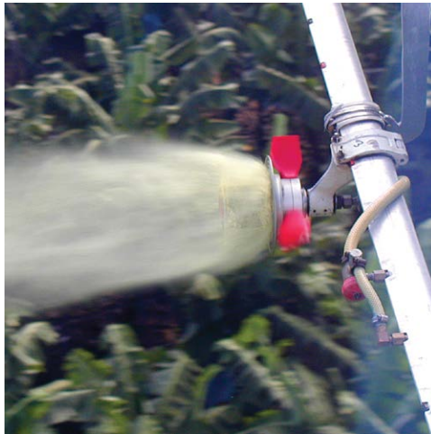
Fig. 5.4. Rotary atomizer used on aircraft to spray bananas. (Photo courtesy of John Clayton at Micron Sprayers, used with permission.)
