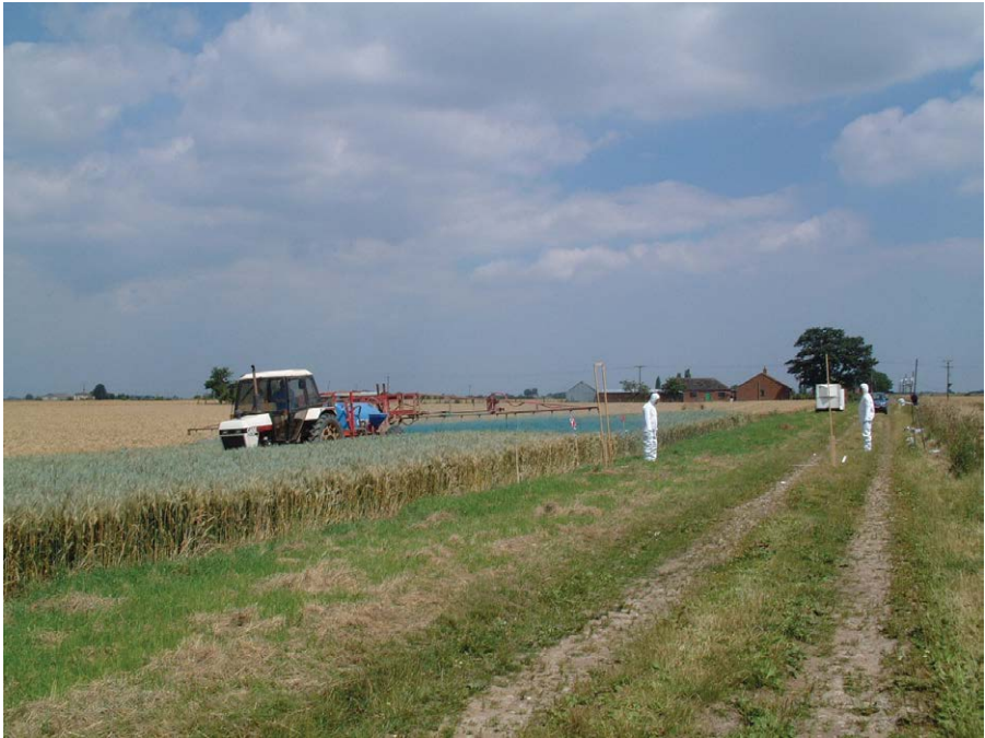
Fig. 9.16. Measuring spray drift downwind from a tractor sprayer in the UK. Bystanders are at the edge of the field with disposable overalls to measure dye collected on different parts of the body. (Photo courtesy of Silsoe Research.)
