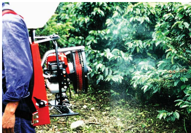
Fig. 5.1. Spraying coffee with a Motax sprayer. (Photo courtesy of Micron, used with permission.)
