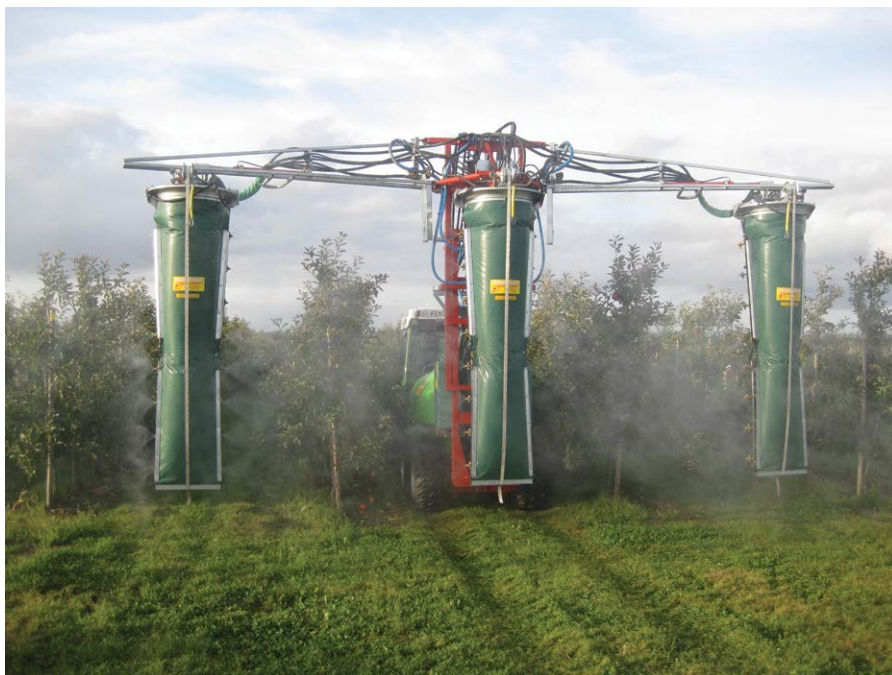
Fig. 2.14c. Modern unit with air-assisted vertical booms to treat multiple rows in an orchard.
