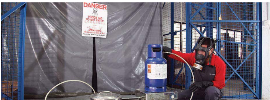
Fig. 6.4. Preparing to add fumigant under the plastic sheeting. (Photo courtesy of Rentkil.)
