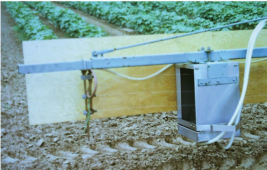
Fig. 4.3. In the USA, straight jets are used to control weeds above a crop.
