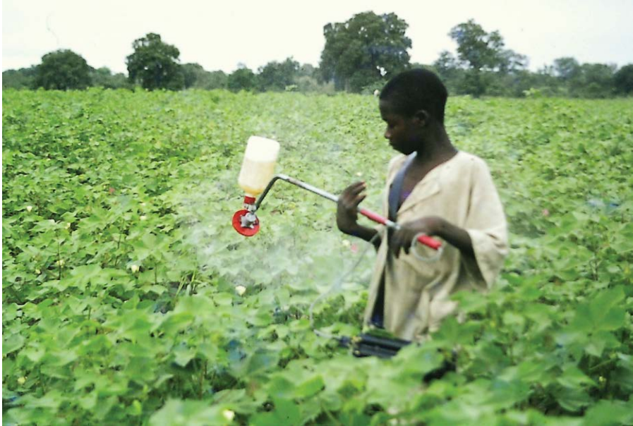
Fig. 2.17a. Early ULV sprayer for treating cotton crops in Africa.
