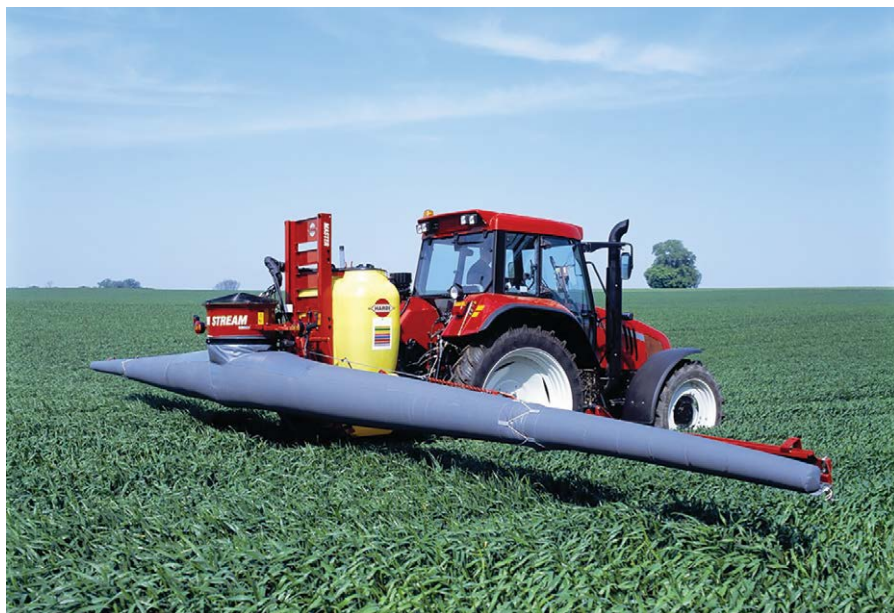
Fig. 2.12. Sprayer boom modified with air-inflated sleeve to project spray downwards into the crop. (Photo courtesy of Hardi.)
