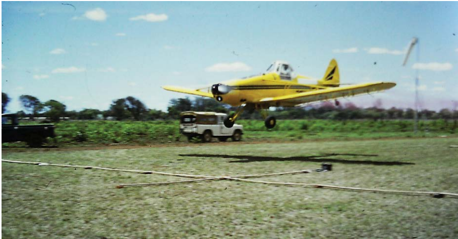
Fig. 2.23d. Aerial spraying – checking swath width with dyed spray.
