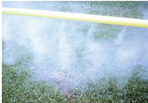
Fig. 2.2b. Adaptation of mistblower with holed long tube. It was used to apply dust on rice in Japan.
