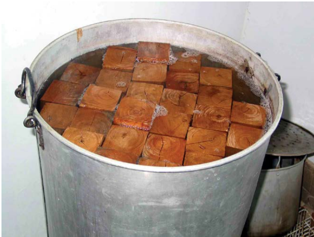
Fig. 5.2. Rubber wood blocks are boiled for 5–7 h.
