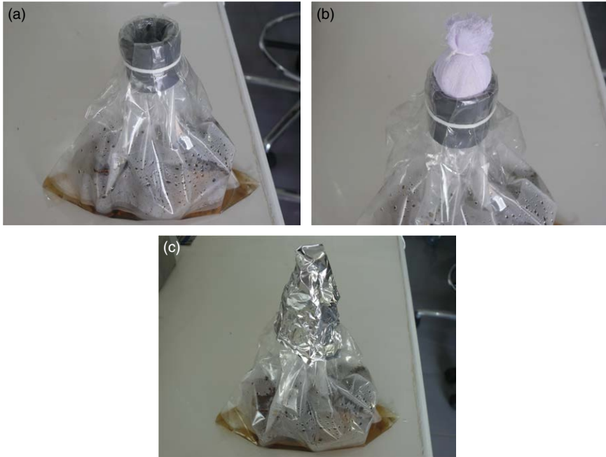
Fig. 5.3. (a) Rubber wood blocks are placed in a PP plastic bag and PA medium added via a PVC pipe through the mouth of the bag. (b) The mouth of the plastic bag is sealed by a stopper. (c) The mouth of the plastic bag is then covered with aluminium foil.
