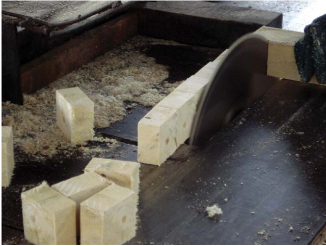
Fig. 5.1. The preparation of rubber wood blocks in a sawmill.
