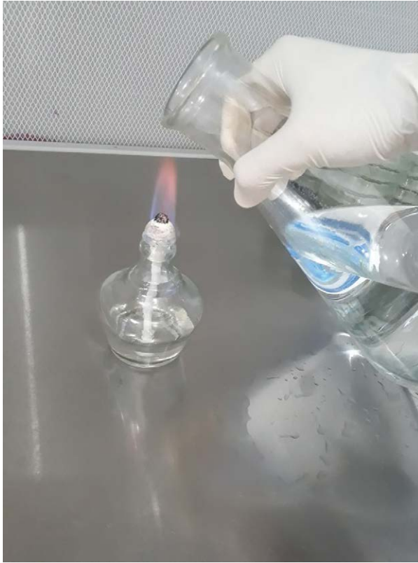
Fig. 3.1. Flaming the mouth of Erlenmeyer flask to sterilize before pouring the medium; training is required to learn this skill.
