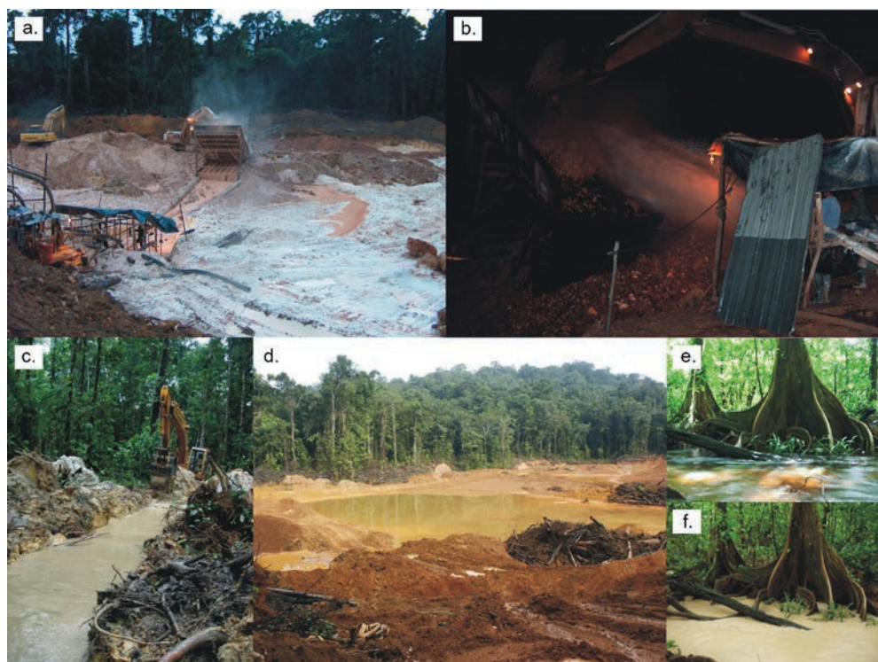
Fig. 9.1. Illustration of artisanal or semi-industrial gold mining activities in French Guiana. From top left to bottom right: (a) mechanical removal of surface soil horizons, (b) stripping off of gold-bearing material with water jets to recover gold particles and nuggets, (c) digging of a derivation canal, (d) settling basin, and water turbidity in Combat Creek (e) before and (f) during artisanal small-scale gold mining activities.
