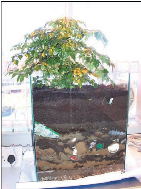
Fig. 7.1. Typical urban ‘Technosol’ profile composed of native soil-forming materials, waste artefacts and organic amendments.
