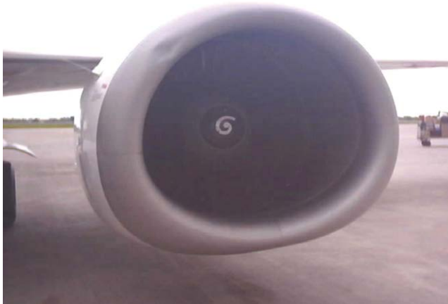
Fig. 9.10. A dent in an aeroplane engine caused by a bird hit. (Courtesy of NAIA, Manila.)
