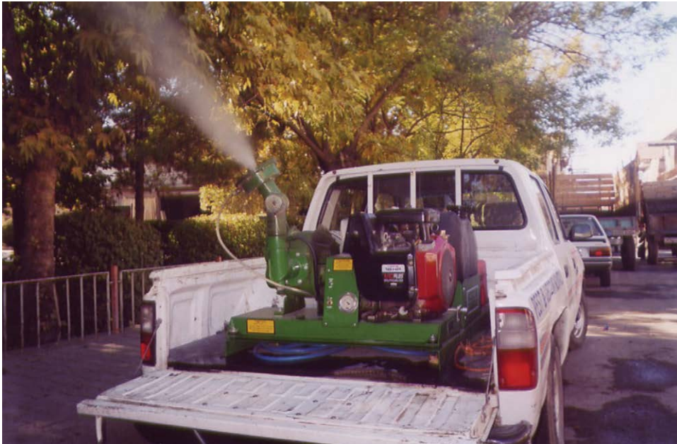
Fig. 4.11. Truck-mounted ULV machines are useful for achieving area-wide coverage in a short time. (Courtesy of Biosav.)
