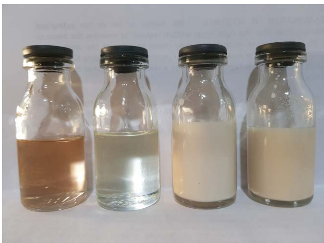
Fig. 10.2. Different forms of liquid formulations (from left to right): emulsion concentrate (EC), Gel, suspension concentrate (SC) and microencapsulation (ME). (Author's picture.)
