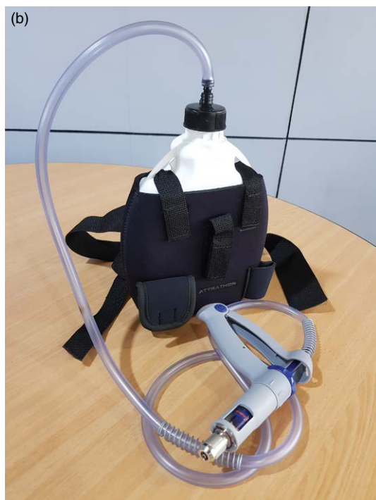
Fig 10.1. (b) A body-wearable plastic sprayer for specialized spraying. (Author's photo.)
