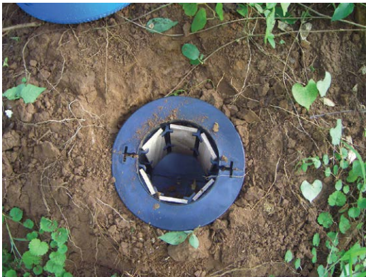
Fig. 11.10. A typical in-ground station with wooden interceptors. (Author's photo.)
