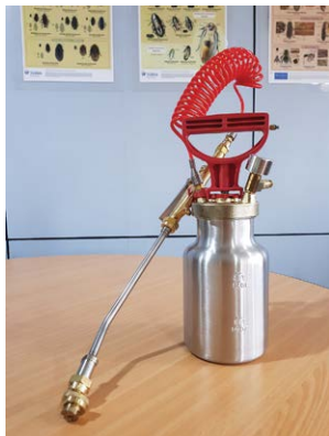
Fig. 10.1. (a) A typical handheld metallic compressed air sprayer. (Author's photo.)
