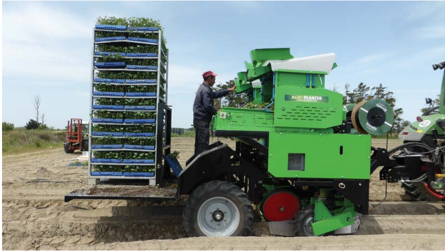
Fig. 12.4. Mechanized planting on sandy alluvial soil in southern France. An automatic vegetable transplanter is pulled behind a tractor and fed with multicell plastic trays (photo: Ph. Vernier).
